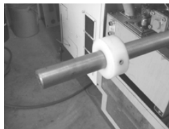
1. Place bar support collar around barstock. Tighten set screw.
