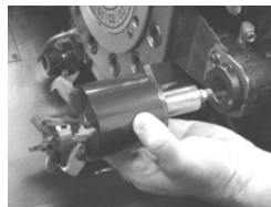
3. Place SBM Bar Puller in tool station.
